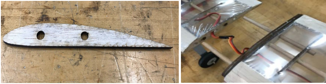
Figure 35: Original wing rib to modified rib to allow wiring to pass through
